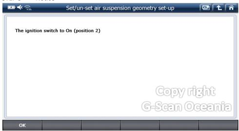
STEP 4 G-scan shows one of four possible displays depending on the vehicle's status.
